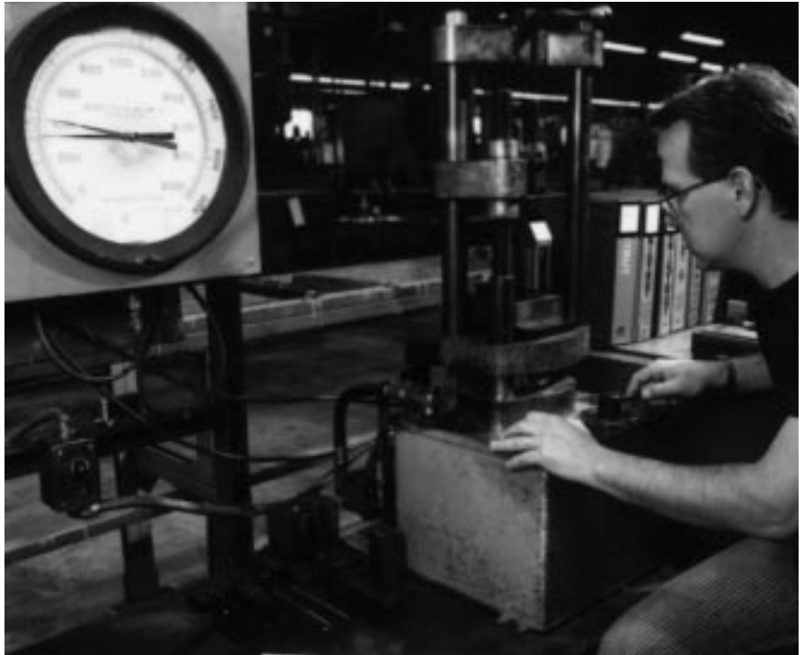
Fixture testing of Unistrut brackets establishes design loads and technical specifications.
